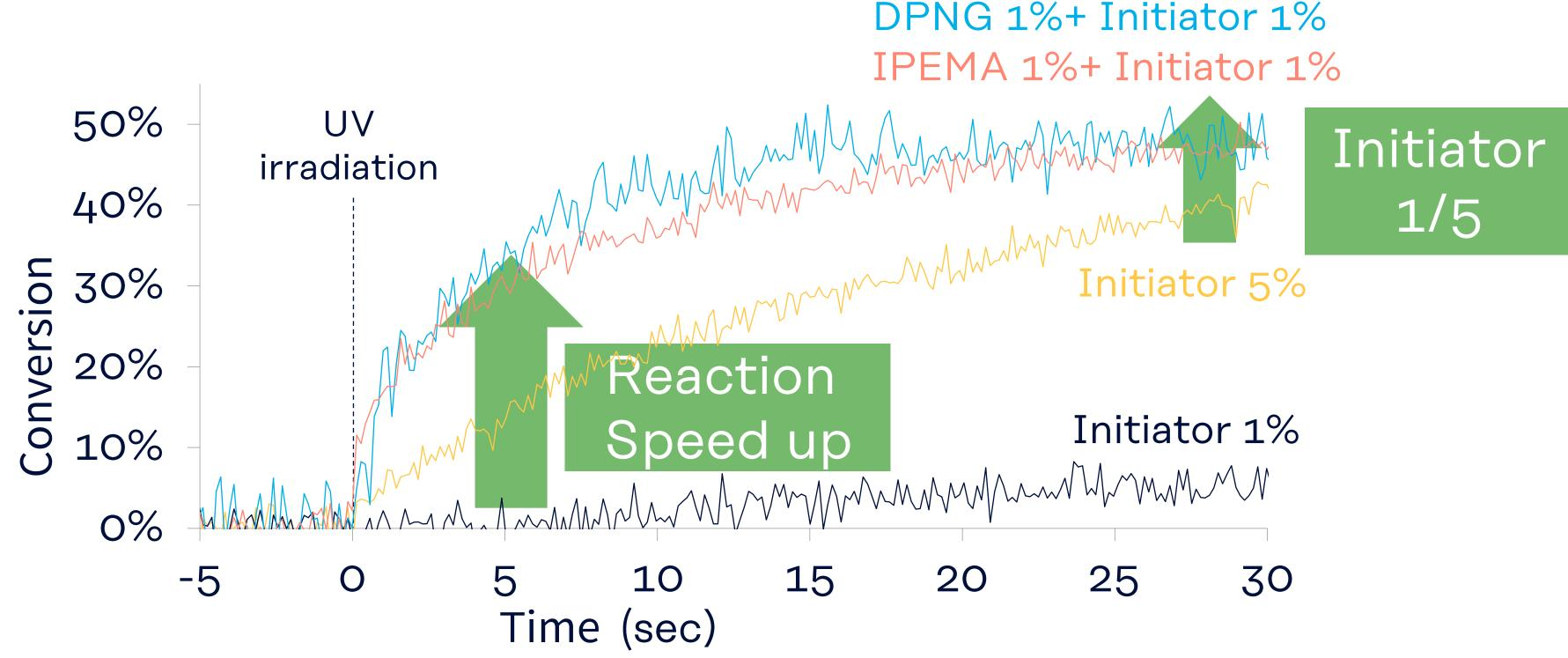
Monomer: Pentaerythritol triacrylate Initiator: 1-Hydroxy-1-cyclohexyl phenyl ketone Thickness: 5µm UV irradiation: 73mW/cm2, high-pressure Hg lamp Atmosphere: Under air Detection: Real-time IR measurement
